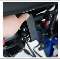
Stand on the side of the wheelchair, press the locker plate with one hand, and push the handle bar toward the seat with another hand.
