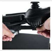
Release the locker and adjust forward or backward.
