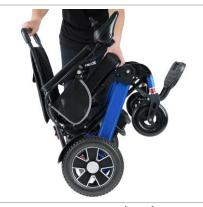
Continue to push the seat downward until you hear a click sound when the spring pin in the middle is inserted into the fixing hole.
