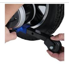
Instert the wheel frame and align the holes on the tubes of anti-tip device and wheel frame.
