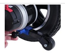
Pull the latch out of the tube of anti-tip device.
