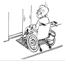
Operator should pay attention to elevator door open and close interval to avoid a collision while enter or exit the elevator, avoid collisions.
