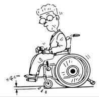
The crossing step should be not higher than 40 mm while normally drive, and have to cross slowly.
