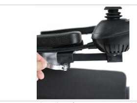
Insert into the tube of arm support and lock.
