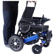
Continue to lift it up until you hear a click sound when the spring pin in the middle is inserted into the fixing hole.
