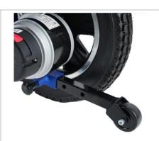
2 positions for adjustment. The installation method is the same for left and right.
