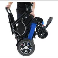
Continue to stand on one side of the wheelchair, hold the handle bar with one hand, grasp the front of the seat frame with the other hand and pull it toward the backrest until the wheelchair is fully folded.
