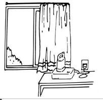
A Battery should be placed in a cool, dry and well ventilated place while charge or store. Has to keep the battery away from fire and heat source, avoid direct sunlight.
