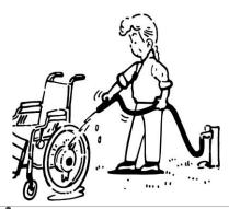
Forbid to use water to rinse this electric wheelchair directly, should use dry or wet cloth to clean, forbid to use corrosive liquid.
