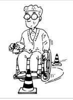
Lightly push the joystick to practice obstacle avoidance, and practice the speed control accordingly.
