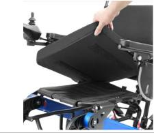
The seat cushion is fixed by Velcro, which is easy to disassemble and assemble.
